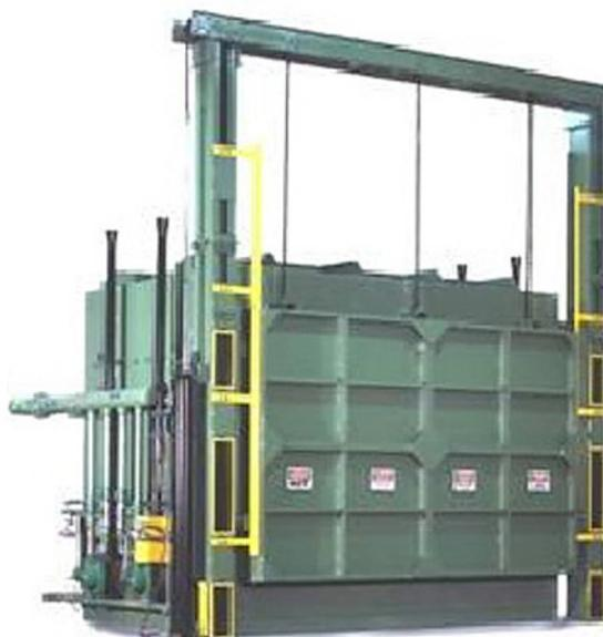
*Side view showing lower TJSR Burners with eductor extensions*
