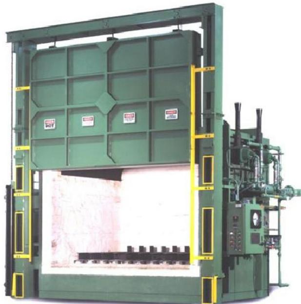
*Front view of the furnace showing the location of the upper TJSR burners.*
